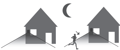
MODE 2 NightGlow with On/Off motion control. Floodlight stays on dimmed setback output until motion switches light to 100% for set dial time.
